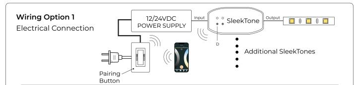
If you are installing more than one Wall Switch unit, all others must be switched Off while pairing.
